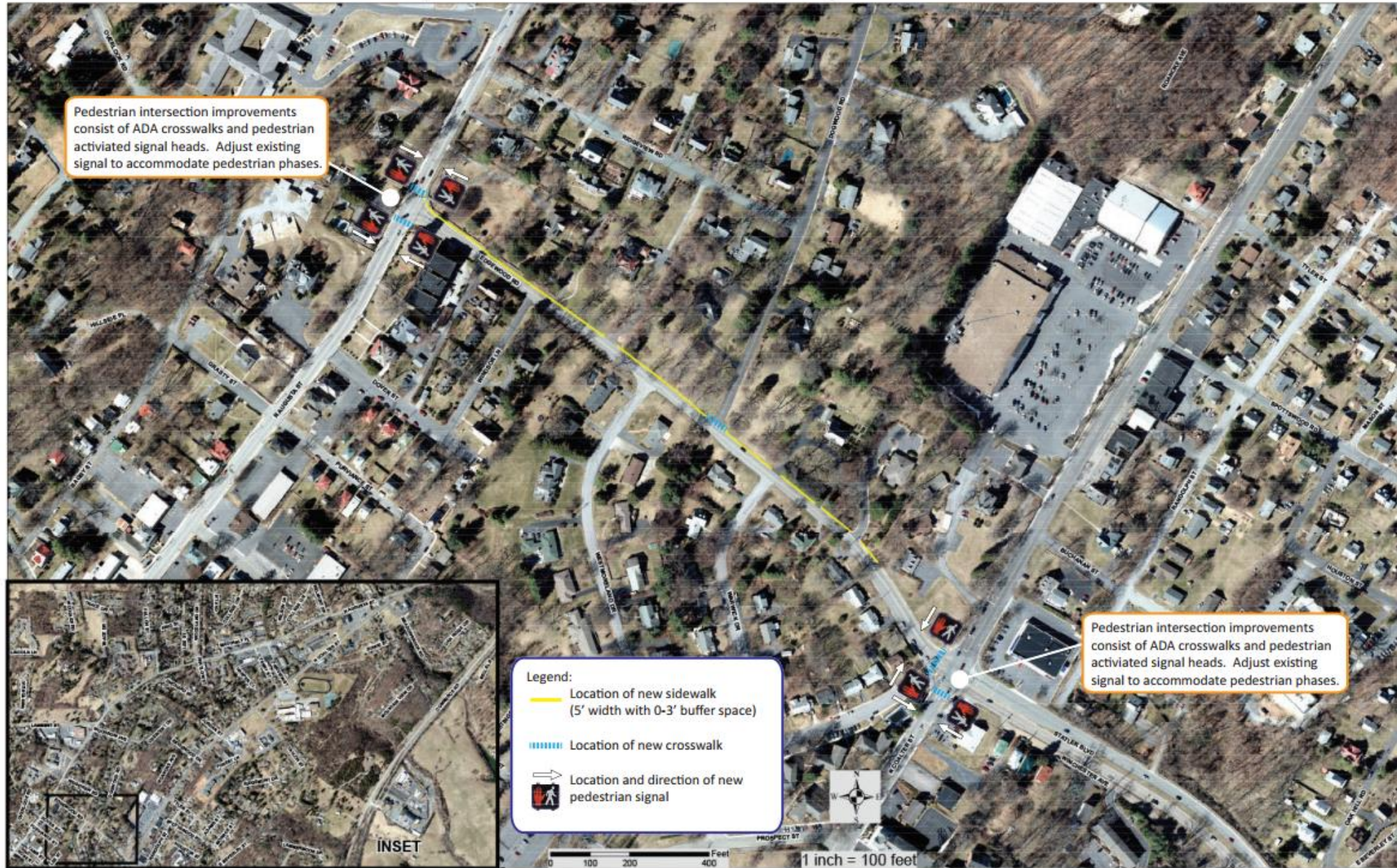
Proposed Sidewalk Improvements to Edgewood Ave.
